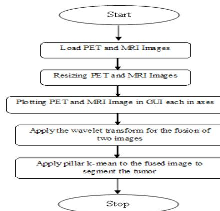
Figure 1: Flow chart of simplification Mat lab program
